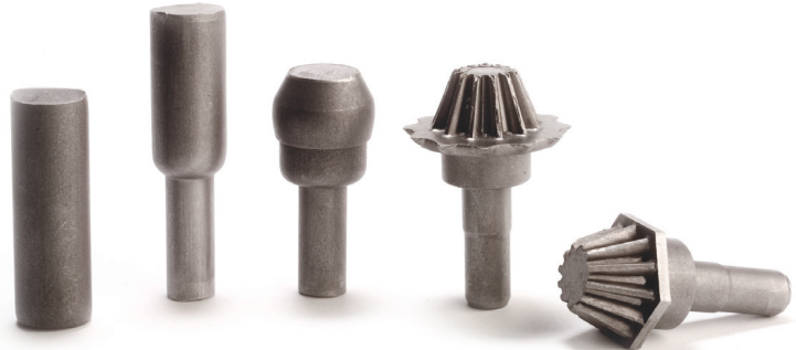
Progressive steps of Cold Heading process
