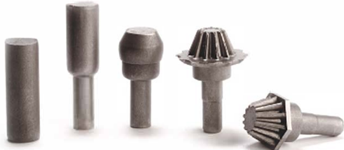
Progressive steps of Cold Heading process
