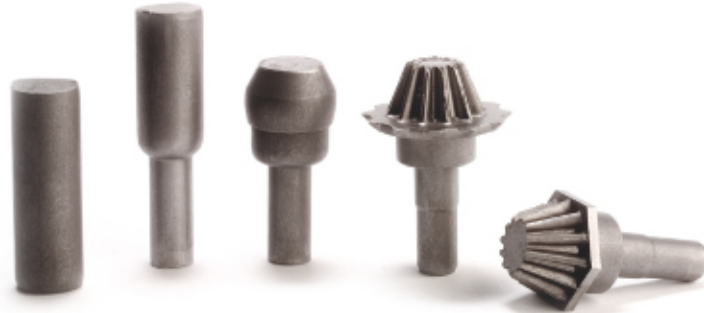
Progressive steps of Cold Heading process
